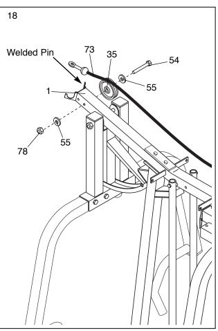
19. Wrap the High Cable (73) around a 3 1/2" Pulley (35) in the direction shown.
